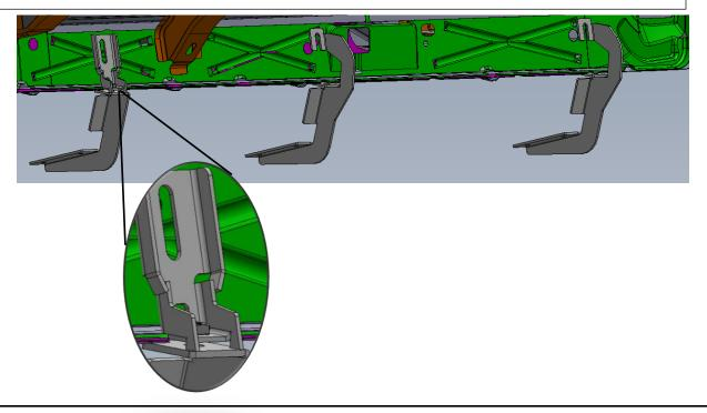
**Step 5:** Set running board along the top of all four brackets and center along the cab.
