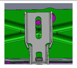
**<u>Step 3</u>**: Using the supplied M8x25mm hex bolts and washers begin hand tightening both upper and lower mounts to the rear two brackets.
