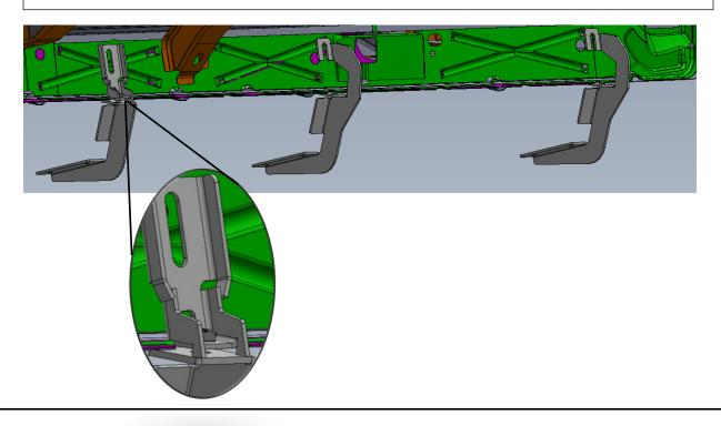
**<u>Step 5:</u>** Set running board along the top of all four brackets and center along the cab.
