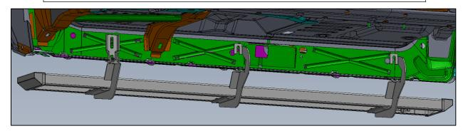
**<u>Step 6</u>**: Insert the supplied threaded brackets (x3) inside the running board lip over the top of each bracket.
