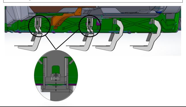
**Step 6:** Set running board along the top of all four brackets and center along the cab.
