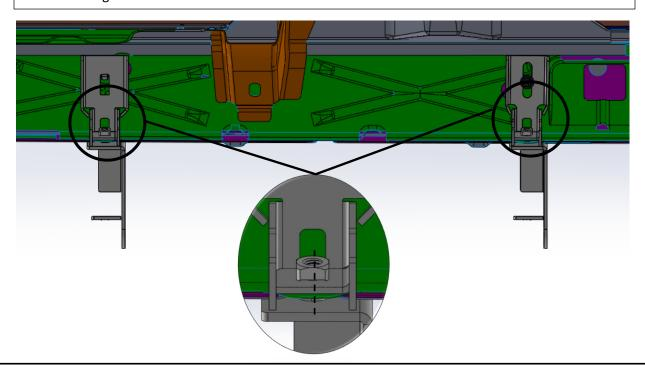
**Step 6:** Set running board along the top of both brackets and center along the cab.
