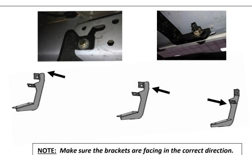
**Step 6:** Set running board along the top of both brackets and center along the cab.
