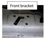
U-clip positioning. <u>NOTE:</u> U- Clip orientation will be the same for passenger
