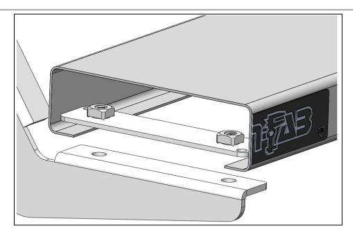
**<u>Step 7</u>**: After final adjustment, tighten all running board threaded mounts. **<u>Step 8</u>**: Next, tighten the lower attachment points (x3).
