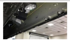
**<u>Step 2</u>**: On the inside rocker panel there will be three 8mm studs coming out from the panel. These studs may be covered in paint and will need to be cleaned before the installation.
