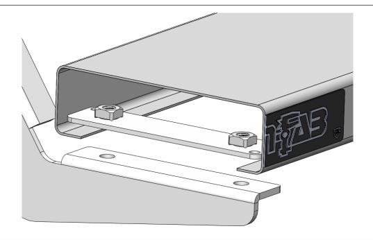
**<u>Step 8</u>**: After final adjustment, tighten all running board threaded mounts. **<u>Step 9</u>**: Next, tighten the lower pinch weld attachment points (x3). **<u>Step 10</u>**: Finish by tightening the upper mounts (x3).
