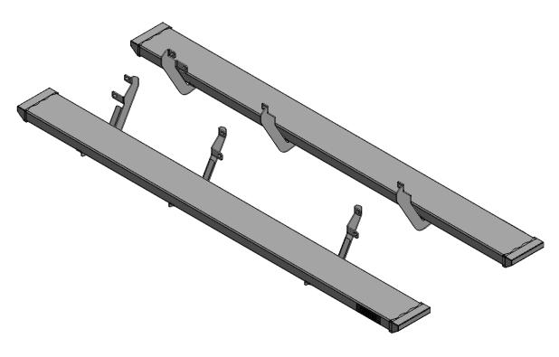
**<u>Step 1</u>**: Starting with the Driver Side. Remove all 8mm flange nuts from the 8mm factory threaded studs to remove the OE running boards. Repeat for passenger side.
