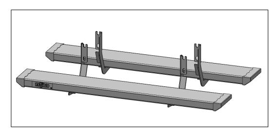
**Step 1:** Starting with the Driver side, locate the holes for the upper mounts (x2) and install the supplied (x2) 3/8" clips in each position. See below for configuration.
