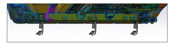
**Step 4:** Set running board along the top of all three brackets and center along the cab.
