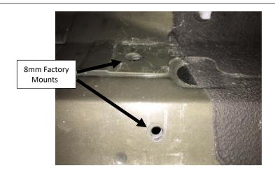
**Step 2:** Starting with the driver's side, install the (x3) rocker panel mounting brackets to the factory attachment points using the supplied M8X30mm Hex Cap Bolt with washer and leave loose at this time.
