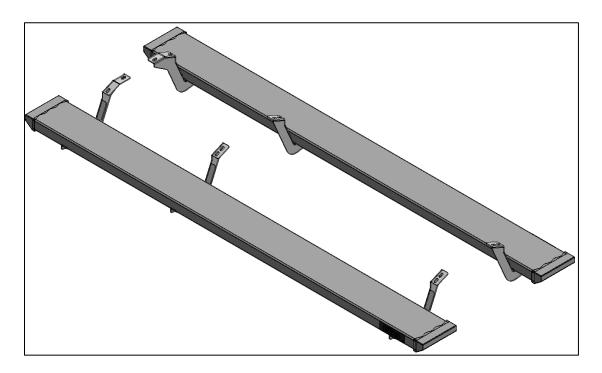
**<u>Step 1</u>** Beginning with the driver side, remove the factory hardware and discard. <u>**Step 2**</u> Next, install the three rocker panel mounting brackets with the supplied M8x25mm Hex bolts with integrated washers and leave loose.
