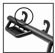
STEP 3: Insert spring loaded U nuts to the body of the truck.
