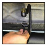
STEP 4 (Drivers Side): Carefully place HS2 step into place. Use bolt, washer and begin hand tightening all 4 upper mountings. Best to have a assistant to lift and hold board in place.
