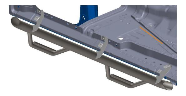
**Step 5:** Next, tighten the three lower bolts first following with the three upper bolts.
