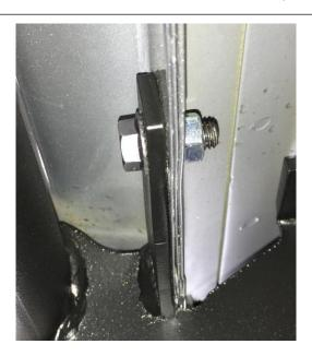
**Step 9.** Next, tighten the remaining hardware that attaches the bracket to the upper body mount.
