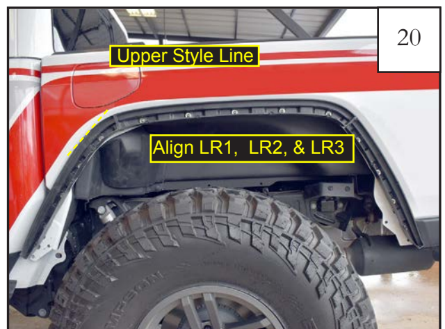
Ensure that inner pieces LR1, LR2, & LR3 are aligned together properly, and tighten all allen head bolts. Inner piece should rest along upper style line of sheet metal radius and not below it.
