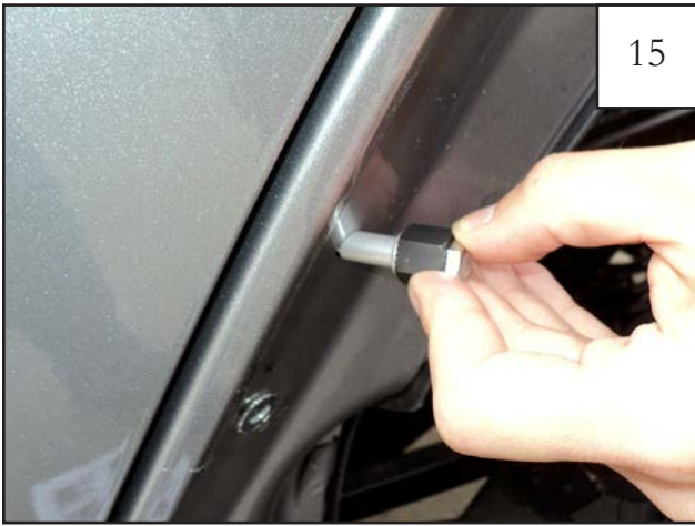
Insert rivnut in fender hole.
