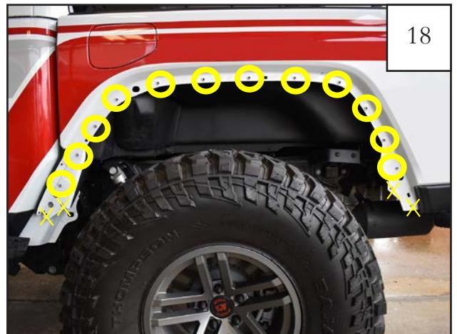
Install (12) rivnuts in rear fender area using the same procedure as Steps 14 thru 17. Test fit inner pieces LR3, LR2, and LR1 (Front to back). NOTE: The "X" above indicates a hole that is not used.
