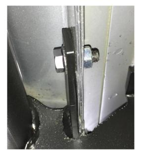
Step 8. Next, tighten the remaining hardware that attaches the bracket to the upper body mount.
