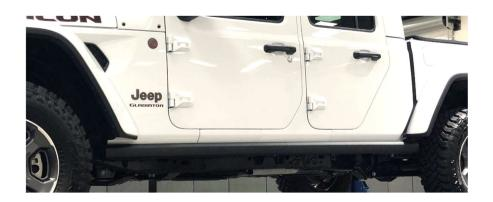
**Step 3.** Carefully raise step up into position and align the brackets with the factory mounting points with the horizontal part of the bracket on the outside of the pinch weld.
