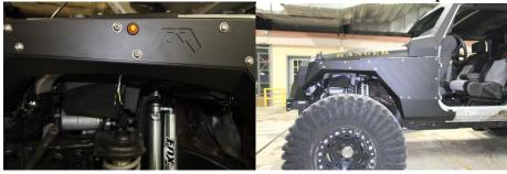
**6.** The fender should be tightened down starting from the back and working your way forward. Be mindful when tightening down the fender bolts as the factory nut clips can be fragile.
