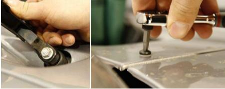
4. Unbolt the fender bolts that are located under the wiper cowl. Note: Remove the factory antenna at this time for passenger side fender removal. Save for reinstallation.
