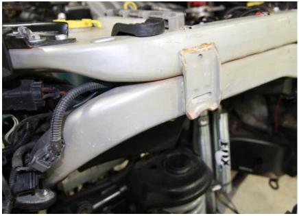
**11.** Reinstall the factory cowl side panels, center cowl panel, and windshield bracket using factory hardware.
