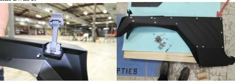
**3.** While the fender is on the floor, install the marker light and grommet to the fender skin. Allow the marker light wires to hang into the wheel well opening.
