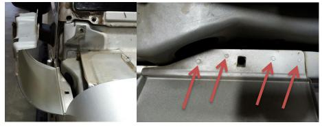
**7.** Using a solid work surface and clamps, clamp the cowl side panel down by the drilled flange and bend the cowl back to original shape. Save the cowl for reinstallation.
