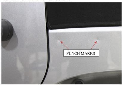
**4.** Once fender is removed, you can begin drilling. Start out by drilling all punch marks with the  $\frac{1}{4}$ " drill bit. Follow behind that with the  $\frac{1}{1}$ 32" drill bit.
