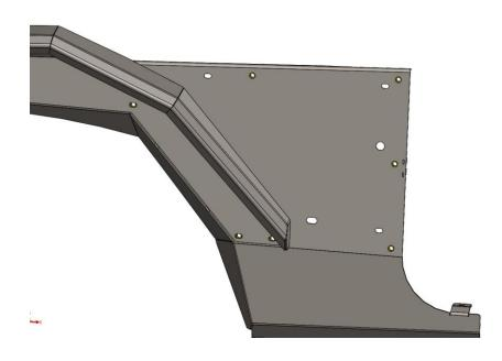
**2.** Position the gill box on the fender base in its mounting position and hand tighten the four 3/8-16 included bolts and washers. The required hardware is supplied in the fender hardware kit.
