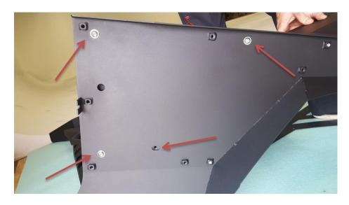
**3.** Align the fender flare and gill box to your liking and fully tighten all hardware.
