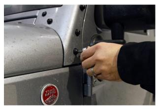
**2.** Remove the four button head torx bolts located in pairs on each side on the factory wiper motor cowl then remove the cowl center.
