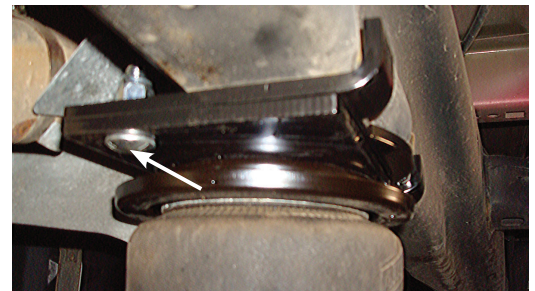
fig. 9b Passenger's side attached with carriage bolts (R), flat washers (M) and nylon lock nuts (U).
