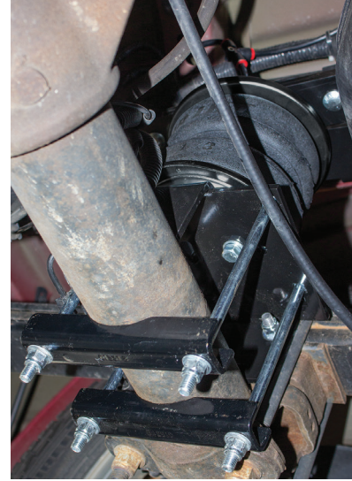
fig. 33 Left (driver's) side: front view of installation.
