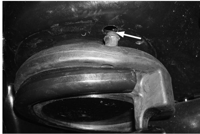
When reinstalling spring assemblies, ensure tab on isolator indexes into the upper spring seat correctly Fig. 8
