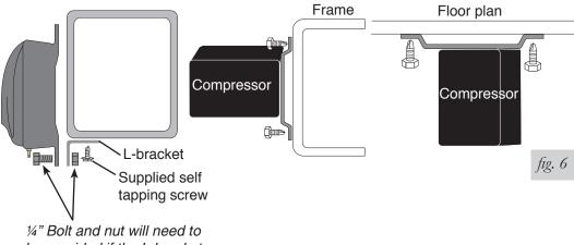
1/4" Bolt and nut will need to be provided if the L-bracket is fabricated.
