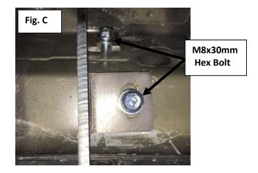
Step 3: Install using the supplied M8x30mm Hex bolt and hand tighten at this time. (Fig. C)
