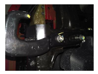
7. Remove the bumper mount brackets from both frame rails using a 14mm socket. Save this hardware for later use.
