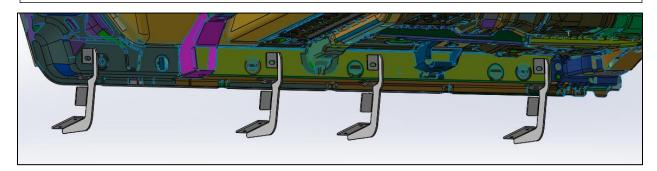
**Step 4:** Set running board along the top of all three brackets and center along the cab.
