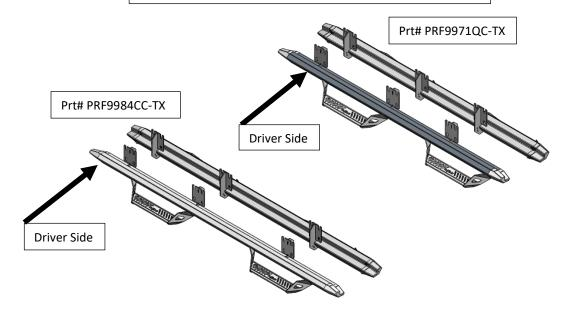
**Step 2** Starting with the Driver side, locate the holes for the upper mounts (x3) and install the supplied (x2) 3/8" clips in each position.
