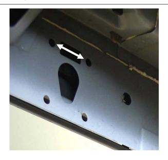
**Step 3** Take the driver side step and carefully raise it up into position and align brackets up to the three mounting positions and start the supplied 3/8" carriage bolts, nuts and washers and hand tighten. **NOTE:** The carriage bolts will start from the outside of the body where the nut and washer will be only visible from the opposite side of the pinch weld.
