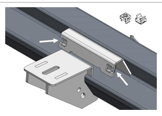
**<u>Step. 4</u>** Carefully raise step rail up to the pinch weld of the body and align brackets up with the factory mounting locations.
