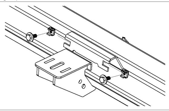
**Step. 7** After finial positioning, tighten all (x6) ¼"x ¾" hex bolts no more than 6 ft/lbs. torque.
