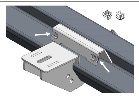
**Step. 4** Carefully raise step rail up to the pinch weld of the body and align brackets up with the factory mounting locations.
