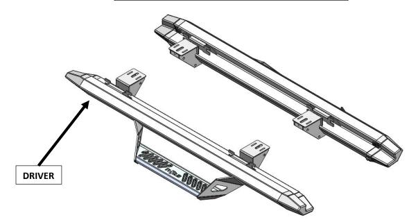
**Step. 2** Starting with the passenger side step rail, install the supplied (x4) 5/16" snap nuts into the two notches in each mounting bracket.
