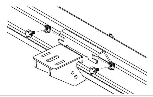
**<u>Step. 7</u>** After finial positioning, tighten all (x4)  $\frac{1}{4}x \frac{3}{4}$  hex bolts no more than 6 ft/lbs. torque.
