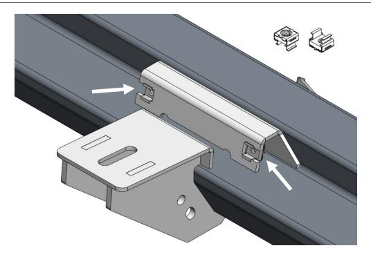
**<u>Step. 3</u>** Carefully raise step rail up to the pinch weld of the body and align brackets up with the factory mounting locations.
