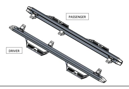
**Step.2** Starting with the passenger side step rail, install the supplied (x4) 5/16" snap nuts into the two notches in each front and rear bracket.
