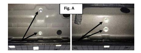
**Step 3** Starting with the driver side, position step up to the body of the vehicle and align the brackets up with the factory mounting locations.
