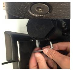
22) Take out the stopper with the threaded end and the two laser cut plates with a + cut into them as shown below.
