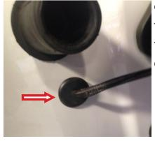
coming out easily, help the rubber fitting from the inside of the tailgate by pushing from the rear and pulling at an angle downward at the same time.
