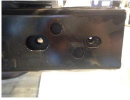
11) Next insert the 4 large 3"x 12mm through bolts through the frame rail with the threads facing the rear of the Jeep, make sure to put the washers onto the bolts as well. NOTE: You'll have to put the head of the bolt above the exhaust canister to get it into the hole.
