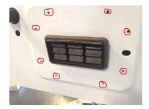
6) Next remove the vent in the middle of the tailgate by gently prying on one of the corners until it pulls out (no bolts/ screws need to be removed) The vent is secured with plastic tabs. Be careful not to break them. Also remove the rubber plug to the right of the vent (circled)
