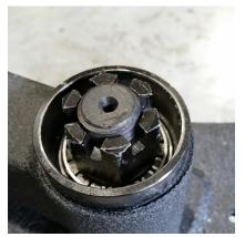
19) Next step is packing the bearings with grease. Once bearing is packed, turn the carrier upside down and place the large bearing in the bottom of the carrier, small side first. Next, install the seal over the bearing by tapping the seal in with piece of wood across it and a rubber mallet. NOTE: It's ok if peels away a little rubber off of the seal when tapping it in.
