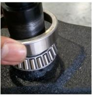
17) Take out your new tire carrier and locate the larger bearing that goes with it. Slide the bearing down the axle with the race facing upward. You may need to sand down the shaft, if the coating is too thick, so you can slide bearing all the way to the bottom of the axle.
