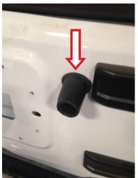
8) Next take the rubber donut and, using the *supplied hardware*, place it on the connector plate as shown in the drilled hole. UPDATE: Use the lower left hole.
