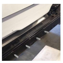
4) Place the spacer plate over the bolts (Not all model bumpers use a spacer plate)
