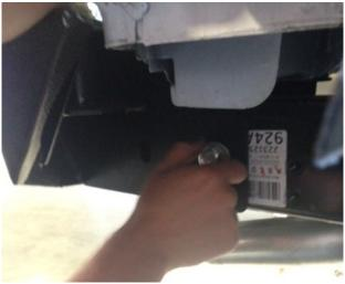
6) Next tighten the through bolts in the rear cross-member first to allow the bumper to properly align itself. Torque to 60 ft/lbs.
