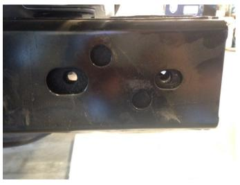
3) Next insert the 4 large 3"x 12mm through bolts through the frame rail with the threads facing the rear of the Jeep, make sure to put the washers onto the bolts as well. (You'll have to put the head of the bolt above the exhaust canister but to get it into the hole but it will fit)
