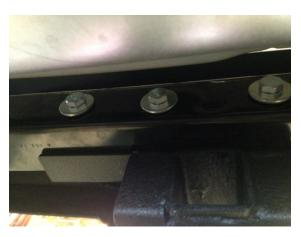
7) Then tighten the 4 side bolts that are loosely inserted into the nut plates. Torque to 60 ft/
