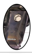
Use supplied M8x30 hex bolts and washers for pinch weld mounts. \*\* From
