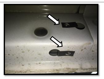
Step 4: Next, remove the front and center body bolts and set aside. Do not remove the bushings.
