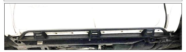
**<u>Step 4</u>** Beginning with the center bracket, start one of the M8x30mm hex bolts into the factory bolt location and leave loose. Start the second M8x30mm hex bolt in the same bracket and loosely tighten.
