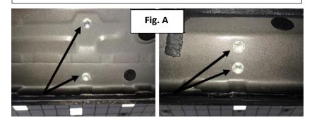
**Step 3** Starting with the driver side, position Trail slider up to the body of the vehicle and align the brackets up with the factory mounting locations.
