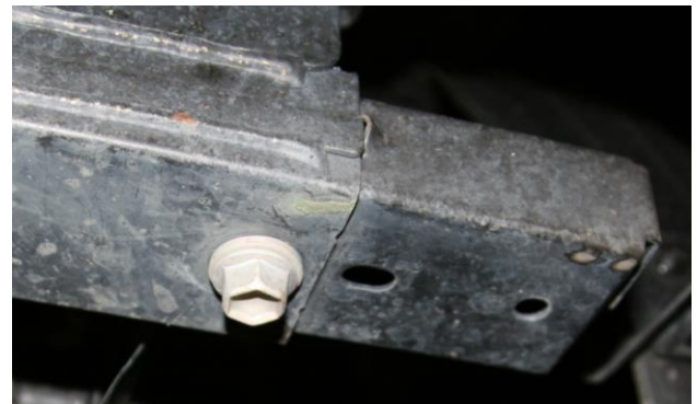
Figure 11 & 12 – Bumper beam extension and tow eye removal
