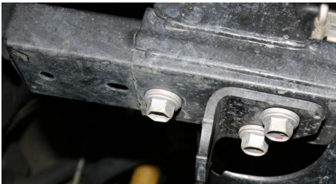
Figure 11 & 12 – Bumper beam extension and tow eye removal
