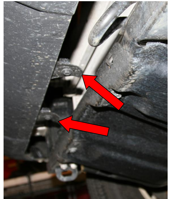
Figure 5 & 6 – OEM bumper cover screw removal
