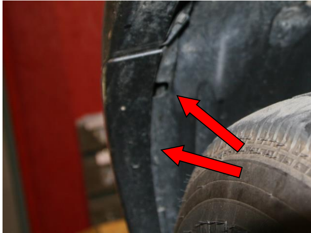
Figure 4 – Fenderwell fastener removal
