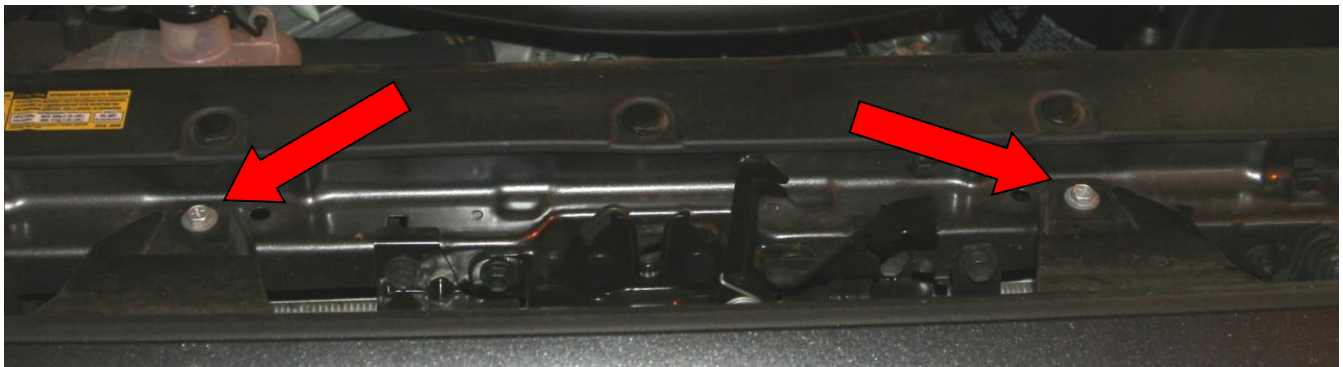
Figure 1 – Upper grill screw removal
