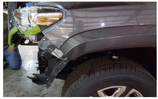
*F.* Mount bumper using OEM 14mm nuts. Do not fully tighten.
