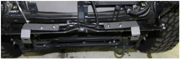
C. With both brackets loosely installed you can now reinstall grill. Once the grill is re-installed, you can fasten the bracket to the grill by lining up the slot on bracket with the cylindrical plastic extrusion on back side of grill and secure the bracket to grill using the provided self-tapping screws.
