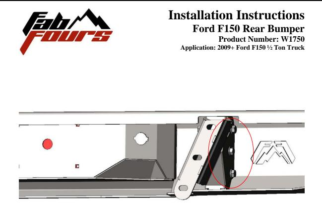
I. Align the bumper from side to side and in and out. Tighten bolts between the bracket and the bumper.
