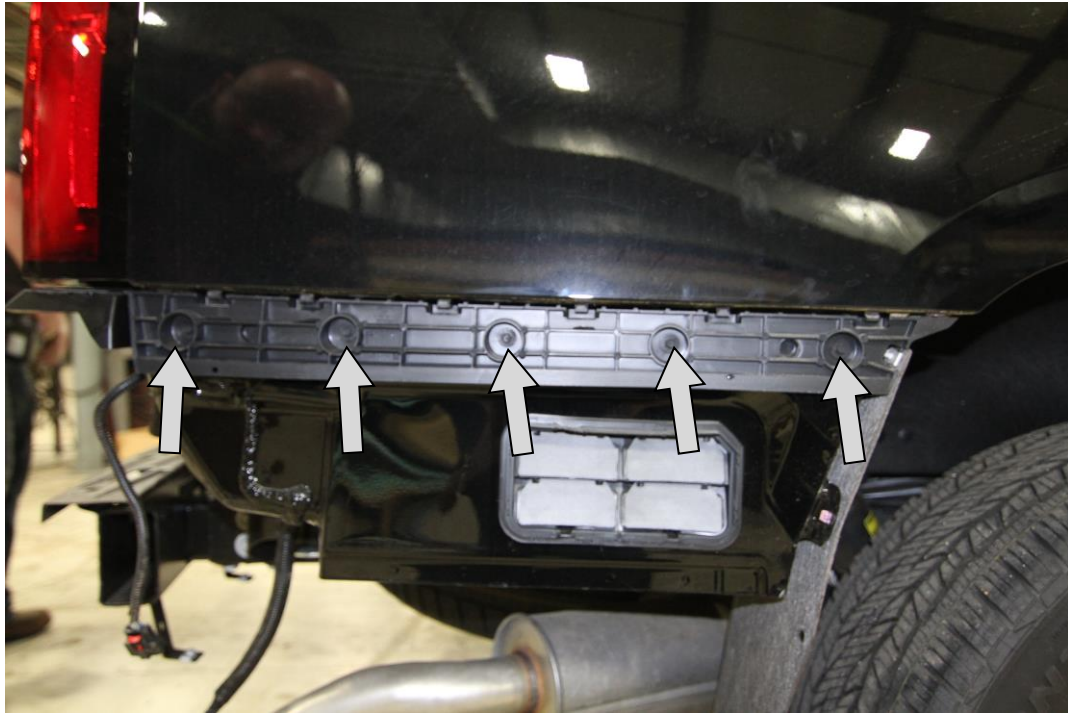
Figure 6 - CLIPPING BRACKET REMOVAL – VIEW FROM BELOW
