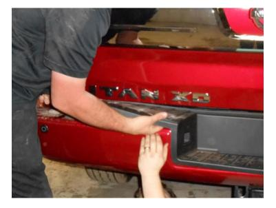
*E.* Remove tailgate by removing the limit straps and camera harness from the bed. Then pull up on the driver's side of the tailgate with the tailgate approximately halfway open. Then slide the passenger side off the pivot point.
