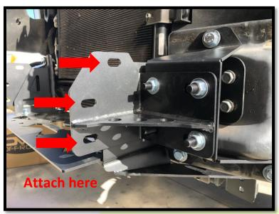
7. Once center section is loosely attached, attach both wings onto center section using supplied hardware. *Ensure to align them with center section* and tighten them down. <u>Do not</u> attempt to line up the entire bumper with body line of truck at this point.
