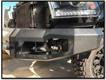
8. Once both wings are attached and fastened securely, locate the wing support brackets. Using provided hardware, attach to this to the inside of each bumper wing loosely and do not attach the opposite side to the truck at this moment.
