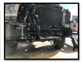
6. Using provided hardware, place center section onto brackets and loosely
