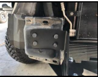
5. Locate and using provided hardware, install main bumper bracket on each side. These are held on by
