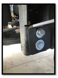
11. Loosely attach skid plate to bumper using supplied hardware. Using the 4" long bolts provided, attach skid plate to backside of frame horn that the winch plate support bracket bolted to. The bolt will be at an angle. You can tighten down at an angle without any damage or integrity loss, or you can open up the hole to level out the bolt. Secure all skid plate bolts.
