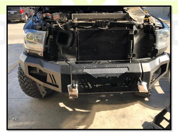
10. Using provided hardware, install the lower bolt for winch plate support bracket. The lower bolt attaches from the front to the inside of the mount on the truck. Secure the bolt on both sides.
