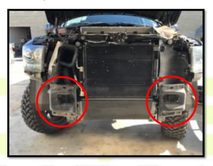
3. Begin by removing the bumper and all of the brackets. Find the two lower winch supports, winch plate, and winch plate mounting brackets. Using provided install hardware, join the three together shown in the below images. Ensure to keep bolts loose for adjustment.
