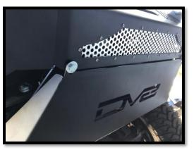
12. Remove front bolt and install wing support bracket reusing factory bolt. Once secured, tighten down <a href="ALL hardware">ALL hardware</a> for bumper. Reinstall factory grill.
