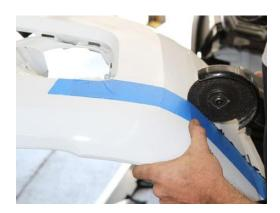
8) After sanding/filing rough cut edges, reinstall the trimmed piece under the headlight (A small gap is normal here)
